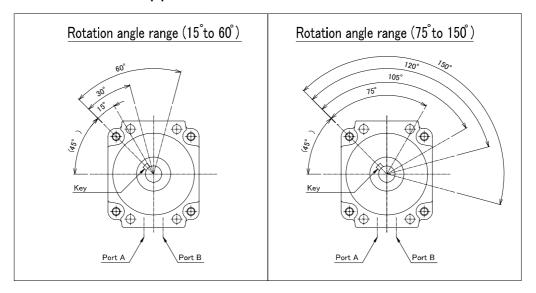
The illustrations above show the key positions when B port is pressurized.
