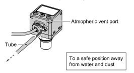
• Insert the tube into the atmospheric vent port until it bottoms out. SMC TU0425 (polyurethane, O.D  $\phi$ 4, I.D  $\phi$ 2.5) is a suitable tubing.
