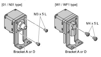
For products with M8 (3 pin) connector, be sure to reserve a space for the lead wire and connector.
