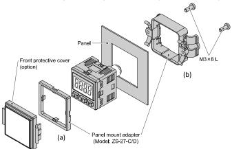
\*: The panel mount adapter can be rotated through 90 degrees for mounting.
