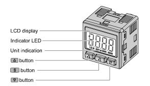
Indicator LED (Green OUT1 and Red OUT2): Displays the switch output condition.
