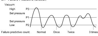
The failure predictive detection counter is incremented when the switch is turned on then is turned off, without the pressure (exceeding P1) not reaching the failure predictive pressure (P3).
