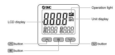
Operation light: Displays the switch operating condition.
