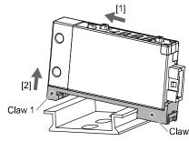
Move in the direction [1], then remove claw 1 in direction [2] as shown.
