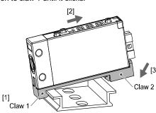
Engage claw 1 of the adapter on to the DIN rail as shown [1], apply force in direction [2], then press downward [3] until claw 2 clicks on to the DIN rail.
