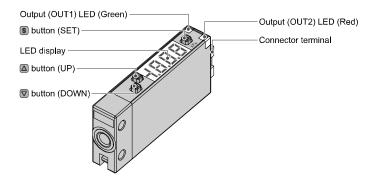
Output (OUT1) LED (Green): LED is ON when the switch output (OUT1)
