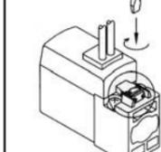
**Caution:** Gently operate using small screwdriver [Torque: 0.1Nm or less]
