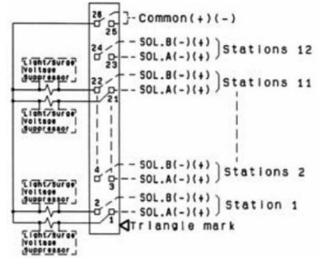
(Note) This circuit shows 2 position double, 3 position, 4 position dual 3-port valve up to 9 stations. The valves are connected in order of 1 → 2 → 3 → 4 so that there will be no extra terminal.
