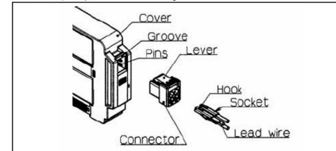
**2. Crimping of lead wires and sockets**
