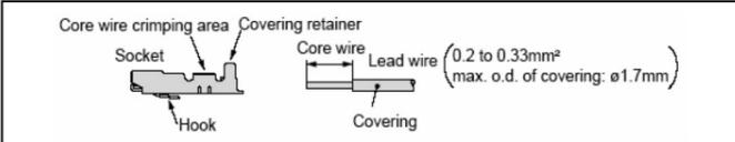
**3. Attaching and detaching lead wires with sockets**
