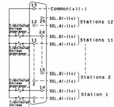
(Note) This circuit shows 2 position double, 3 position, 4 position dual 3-port valve up to 12 stations. The valves are connected in order of 1 → 14 → 2 → 15 so that there will be no extra terminal.
