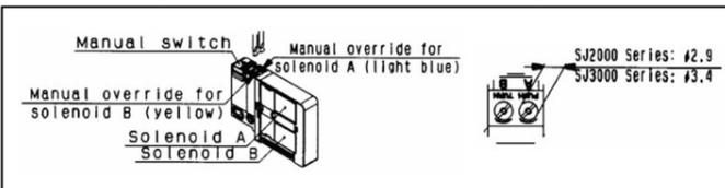
With D type, use a precision driver (flat blade) and rotate lightly. [Torque: Less than 0.1Nm] When D type is locked, be sure to push before rotating. Rotating without pushing may break manual override and cause failure such as air leakage.
