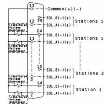
(Note) This circuit shows 2 position double, 3 position, 4 position dual 3-port valve up to 12 stations. The valves are connected in order of 1 → 14 → 2 → 15 so that there will be no extra terminal.
