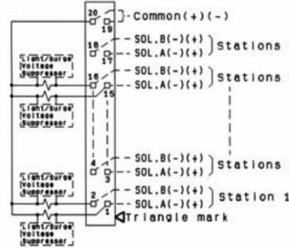
(Note) This circuit shows 2 position double, 3 position, 4 position dual 3-port valve up to 12 stations. The valves are connected in order of 1 → 2 → 3 → 4 so that there will be no extra terminal.
