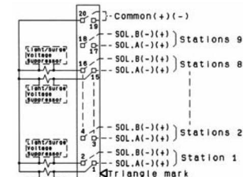
(Note) This circuit shows 2 position double, 3 position, 4 position dual 3-port valve up to 12 stations. The valves are connected in order of 1 → 2 → 3 → 4 so that there will be no extra terminal.
