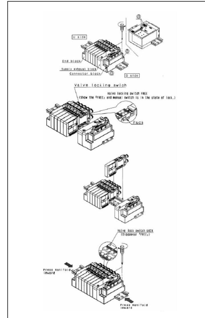
1. Loosen screws a fixed to DIN rail (2pcs at one side)
