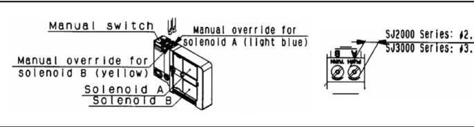
With D type, use a precision driver (flat blade) and rotate lightly. [Torque: Less than 0.1Nm] When D type is locked, be sure to push before rotating. Rotating without pushing may break manual override and cause failure such as air leakage.
