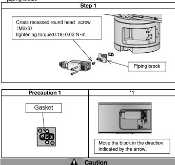
• When installing the gasket on the piping block, pay attention not to have dirt attach to it.
