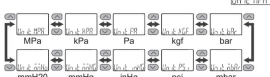
\*: The unit that can be displayed is different depending on the pressure range. (kPa/MPa/Pa can still be selected if the product does not have the units selection function.) Refer to the operation manual, available from the SMC website (URL <http://www.smcworld.com>) for more detailed information.
