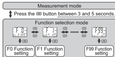
\*: Some products do not have all the functions. If no function is available or selected due to configuration of other functions, [- -] is displayed on the sub display (right).
