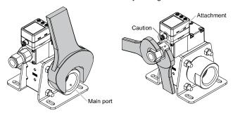
After hand tightening, apply a spanner of the correct size to the spanner flats on the product, and tighten it for 2 to 3 rotations, to the tightening torque shown in the table below.
