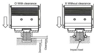
· Stroke end when turning over
