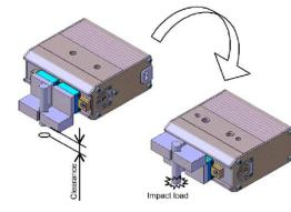
• When mounting a work piece, align it with the product carefully to prevent excessive force being applied to the finger. In particular, during a trial run, operate the product manually or at a low speed and check that safety is assured without impact.
