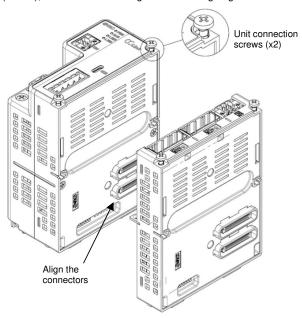
(2) Press down the unit connection screws (2 places) and tighten the
