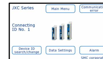
\*If communication cannot be established, check that the Device ID has not been changed to anything other than 1 and that there is nothing wrong with the communication cable, then press the Start Search button, without changing the default setting for the device ID No. (1) on the JXC series device ID setting screen.
