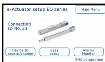
\*If communication cannot be established, check that the device ID has not been changed to anything other than 33 or that there is nothing wrong with the communication cable, then press the Start Search button, without changing the default setting for the device ID No. (33) on the EQ series device ID setting screen.
