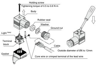
Figure 8. JSP20 DIN connector construction
