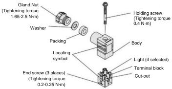
Figure 7. JSP10 DIN connector construction
