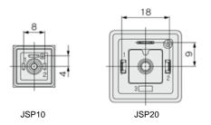
Figure 10. DIN terminal type (conforming to DIN EN 175301-803)
