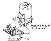
Figure 3. Bracket installation
