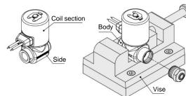
Figure 1. Example of clamp area of valve
