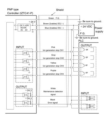
When an ionizer (IZT41/IZT43) is used in DC mode, make sure to ground the F.G. cable (green) and DC(-) cable (blue) of the input power supply with a resistance of 100 ohms or less. Without grounding the DC(-) cable, this products and/or power supply may be damaged.
