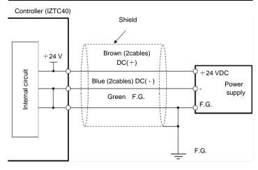
When the product is used in DC mode, make sure to ground the F.G. cable (green) and DC(-) cable (blue) of the input power supply with a resistance of 100 ohms or less. Without grounding the DC(-) cable, this products and/or power supply may be damaged.
