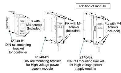
c. Connect the controller and high voltage power supply module
