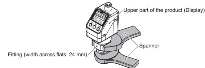
When tightening, do not hold the product body with a spanner.
