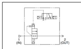
The intended use of IBV series is for use in blowing applications that require high peak impact pressure.
