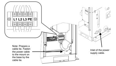
\* Connect over current protection to the power cable connected to the equipment in order to avoid hazard.
