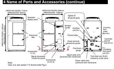
Fig.1: HRSH\*\*\*-A\*-\*\* (Air cooled type)
