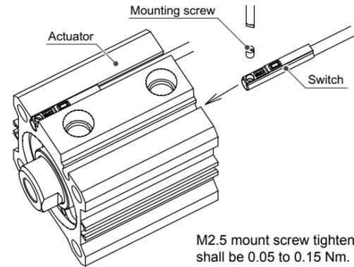
M2.5 mount screw tightening torque shall be 0.05 to 0.15 Nm.
