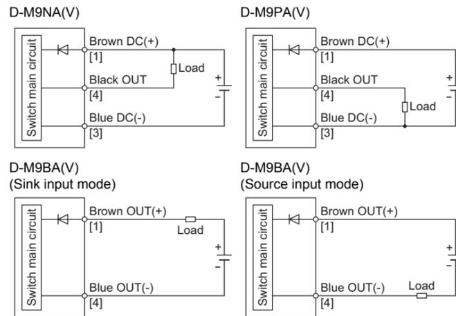
The number shown in brackets [ ] in the circuit diagram indicates the connector pin number.
