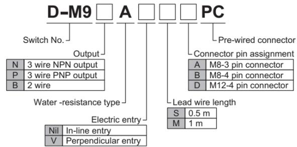
This product is a Solid State Auto Switch of direct mounting specification. Switch should only be used in areas in which potentially explosive atmospheres are unlikely to be present or only present for short periods of time.
