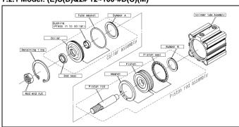
7.2.2 Models: (E)C(D)Q2B 125~200-#DC(M), (E)C(D)Q2# 32~100-#DC(M) / Long Stroke type
