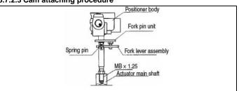
Install positioner feedback shaft and rotary actuator main axis so that they are concentric. Ensuring that the spring pin of the feedback shaft end can enter the end of the fork lever assembly axis.
