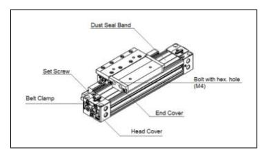
Disassemble the cylinder, remove the old grease and place all the parts on a clean cloth in a clean environment. The following flat head screwdriver or hexagon socket wrench shall be used to loosen the set screws:
