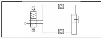
Plugging one of the ports on the actuator is considered a non-intended use, and could relate to an increase in maximum surface temperature above what the product specification declares.
