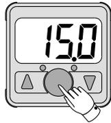
Press the "SET" button for more than 2 seconds until "1no" is displayed. Release it when the display turns to "1nc".
