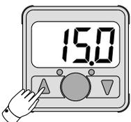
While displayed, pressing the ▲ button for 1 second or longer causes the peak mode to display and blink. Pressing the ▲ button once again for 1 second or longer reinstates it.
