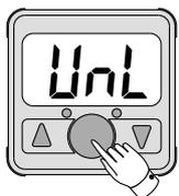
Press the "SET" button for 4 seconds or longer. Release it when the display turns to "UnL".
