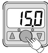
Select the Auto preset mode in the initial setting mode and press the "SET" button until "RP1" is displayed.
