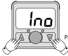
Select the "output mode" for OUT1 by pressing either ▲ button or ▼ button.
