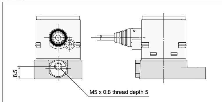
\* For splash proof use (IP65), insert an air tube into the atmospheric release port.
