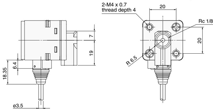
\* For splash proof use (IP65), insert an air tube into the atmospheric release port. (Refer to "Precautions" on page 16-2-24 for details.)
