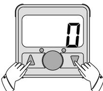
Pressing the ▲ + ▼ buttons simultaneously with the supply pressure released to the atmosphere, causes it to reset to zero on the display and completes the zero clear operation. The function then returns to the measurement mode.
