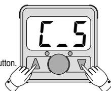
※ Only for ZSE40(F)/ISE40-□-30/70(L)-M, displays the input mode "C\_5" and the compensation value alternately. If auto shift input is not complete, zero is displayed.
