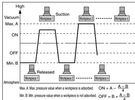
Supplies vacuum pressure, changing the condition of a workpiece by adsorption nozzle, etc. When setting OUT2 is not required, press both the ▲ button and ▼ button simultaneously in this state to skip to the measurement mode.
