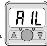
Repeat adsorption and non-adsorption several times in this state. The optimal set value is determined automatically.
