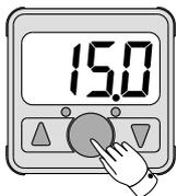
Select the manual set mode in the initial condition mode and press the "SET" button until "P\_1" or "P\_2" is displayed.
