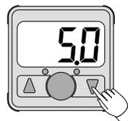
While displayed, pressing the ▼ button for 1 second or longer causes the bottom mode to display and blink. Pressing the ▼ button once again for 1 second or longer reinstates it.
