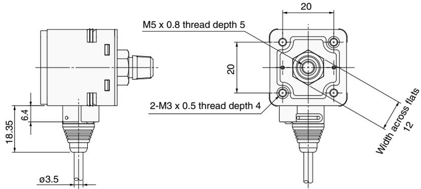
\* For splash proof use (IP65), insert an air tube into the atmospheric release port. (Refer to "Precautions" on page 16-2-24 for details.)
