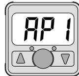
Prepare the equipment for use under operating conditions. When setting OUT1 is not required, press both the ▲ button and ▼ button simultaneously in this state to skip to "RP2".
