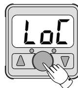
Press the "SET" button for 4 seconds or longer. Release it when the display turns to "LoL".
