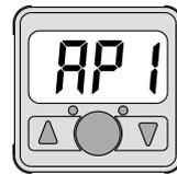
Prepare the equipment for use under operating conditions. When setting OUT1 is not required, press both the ▲ button and ▼ button simultaneously in this state to skip to "RP2".
