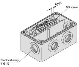
Step 3. How to replace the terminal block cover
