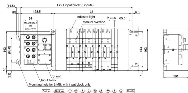
$Formulas: L1 = 25n + 106, L2 = 25n + 241 \ (For \ 1 \ input \ block. For \ each \ additional \ input \ block, \ add \ 54 \ mm.) \ n: \ Stations \ (Maximum \ 16 \ stations)$
