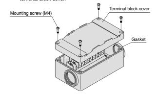
Step 3. How to replace the terminal block cover
