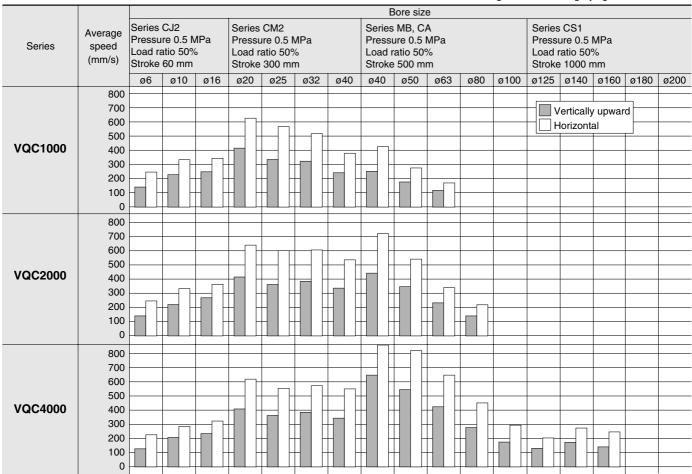
\* Values at extension of a directly coupled cylinder when meter-out speed controllers are used with the needle full open.
