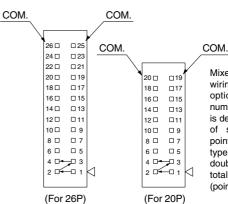
Mixed single and double wiring are available as options. The maximum number of manifold stations is determined by the number of solenoids. Count one point for a single solenoid type and two points for a double solenoid type. The total number of solenoids (points) must not exceed 24.
