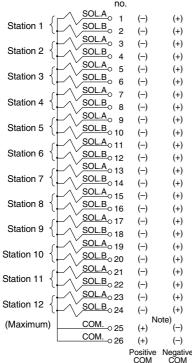
Note) When using the negative COM specification for VQC1000/2000, use valves for negative COM.
