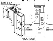
Slide the manual override button with a small flat head screwdriver or with your finger until it stops at the pilot valve side (ON side) to lock it. Slide it to the fitting side (OFF side) to release it. It can also be used as a type using a screwdriver, etc., of ø1.7 or less in case of VQC1000, ø2 or less in the case of VQC2000.
