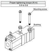
The bushing may be damaged if the tightening torque of 0.8 N·m is exceeded. In the event that damage does occur, be sure to replace the bushing.
