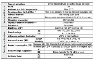
Note 1) Based on dynamic performance test, JIS B 8374-1981. (Coil temperature: 20°C, at rated voltage, without surge voltage suppressor).
