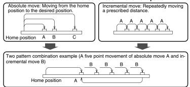
Eight speed patterns based on the speed number and acceleration number can be set, and a speed pattern can be selected for each movement pattern.
