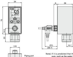
02: Rc1/4 N02: NPT1/4 F02: G1/4 (ISO 1179) Note) If it is predicted that the pressure, such as the water hammer or surge pressure fluctuates rapidly, refer to the Handling Precautions stated in the Operation Manual at SMC website (http://www.smcworld.com).
