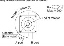
Start of rotation is the position of the chamfer (keyway) when B port is pressurized.
