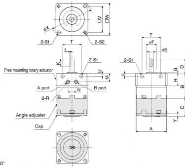
\* Illustrations above show actuators for  $90^{\circ}$  and  $180^{\circ}$ when B port is pressurized, and they show size 20 actuators.
