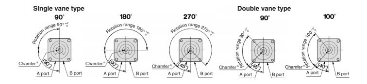
\* For size 40 actuators, a parallel keyway will be used instead of chamfer.
