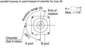
Start of rotation is the position of the chamfer (keyway) when B port is pressurized.
