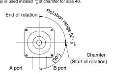
Start of rotation is the position of the chamfer (keyway) when A port is pressurized.
