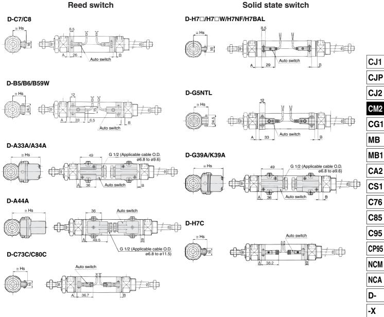
Proper Auto Switch Mounting Position (Detection at stroke end) and Its Mounting Height
