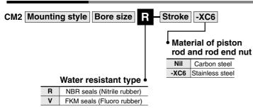
Ideal for use in a machine tool environment exposed to coolant mist. Also suited for use in areas in which water splashes, such as food processing equipment or car washers.
