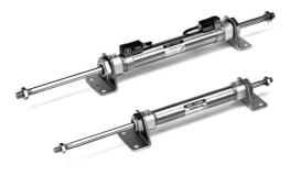
Bore size (mm) 20 25 32 40 Action Double acting, Double rod Fluid Air Proof pressure 1.5 MPa Maximum operating pressure 1.0 MPa Minimum operating pressure 0.08 MPa Without auto switch: -10 to 70°C (No freezing) With auto switch: -10 to 60°C (No freezing) Ambient and fluid temperature Lubrication Not required (Non-lube) Thread tolerance JIS Class 2 <sup>+1.4</sup> mm Stroke length tolerance Piston speed 50 to 750 mm/s Cushion Rubber bumper 0.27 J 0.4 J Allowable kinetic energy 0.65 J 1.2 J
