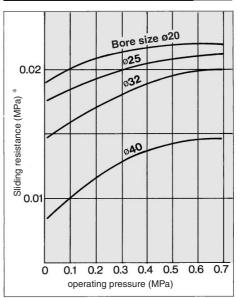
\* Conversion into the cylinder operating pressure: 1 MPa = 10.1972 kgf/cm<sup>2</sup>
