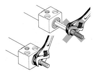
2. When replacing rod seals, please contact SMC. Air leakage may be happened, depending on the position in which a rod seal is fitted. Thus, please contact SMC when replacing them
