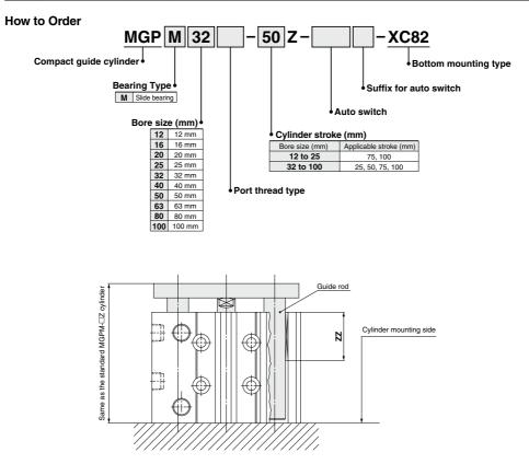
Note) The total length (ZZ) of the guide rod bushing is shorter than the standard type.
