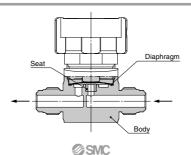
Diaphragm Valve for Ultra High Purity Manually operated type AZ3652 & 4652 Series
