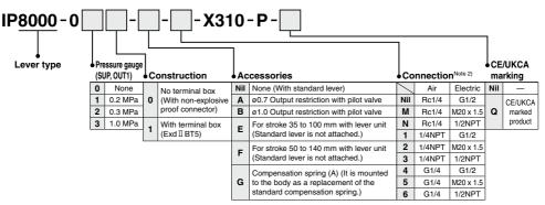
Note 1) If two or more accessories are required, the part numbers should be given in alphabetical order. Note 2) If 1 is selected for Construction, M, N, 2, 3, 5, 6 cannot be selected for Connection.
