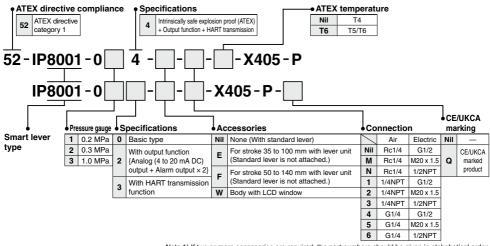
Note 1) If two or more accessories are required, the part numbers should be given in alphabetical order. Note 2) If a connecting port is  $M20 \times 1.5$ , a blue cable gland is included.
