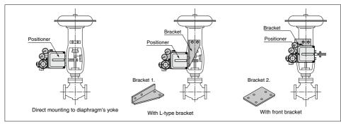
The feedback lever that detects the displacement of valve stems should be mounted at a position so that the lever is at right angles to the valve stem for an input current of 50%. The figure is the configuration viewed from the front.
