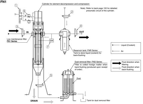
The products indicated in the table below refer to coolant related products. The SGC and VNC series coolant valves Example of Connection Device (with bodies made of cast iron) cannot be used with any fluids (such as industrial water) other than coolant.
