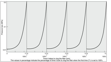
Introduce a certain concentration of dust and back-flush the filter when the pressure loss reaches 0.2 MPa. Repeat filtering and back-flushing process (up to five times shown in the graphs).
