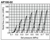
Note) The graph above shows the relief flow when the set pressure rises and falls from 0.1 MPa.
