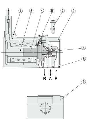
(The normally closed valve is shown.)
