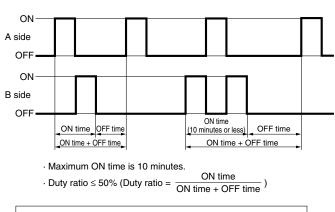
Example: When energization lasts for five minutes, it should be followed by five or more minutes of de-energization. Because the latching type has only one solenoid, both the A side and B side should be off for five minutes or more.
