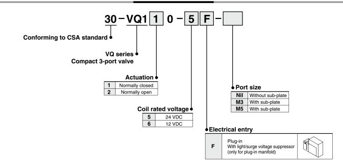
Function: Standard (1 W) Manual override: Non-locking push type (Tool required) Latching type: Push-locking type (Tool required)
