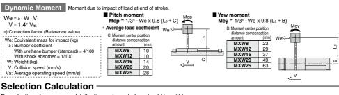
For selection of a proper model, the items shown below should be within the operating range of the graph. Furthermore, find load factors ( $\alpha$ n) and make sure that their sum total ( $\Sigma \alpha n$ ) does not exceed 1.
