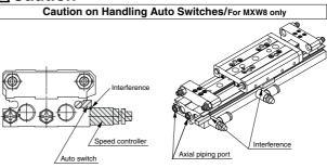
When an auto switch is installed on the port side of MXW8, some switches could interfere with the speed controller or a fitting. Therefore, use one of the methods described below for installing the auto switch.
