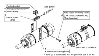
internal side (contact side with the tube).
