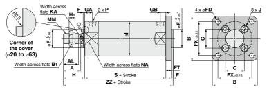
\* End boss is machined on the flange for øE.
