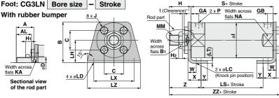
\*1 The rod end nut should be mounted in the position t (clearance) so that it will have a clearance of 1 mm or more in order to prevent interference of the nut with the bolt for mounting bracket when the rod is retracted.
