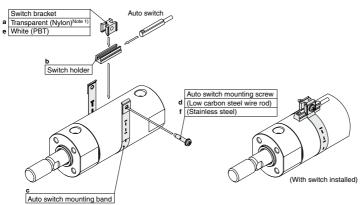
\* Band (c) is mounted so that the projected part is on the internal side (contact side with the tube).
