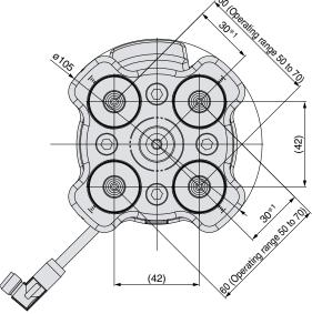
\*1 Operating range: 25 to 35 (When a cup is mounted in the center) As interference between cups may occur depending on the cup diameter, select the cup diameter according to the pitch to be used.
