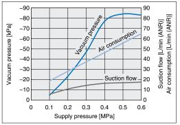
\*1 The exhaust characteristics are different when the vacuum-saving valve (ZP2V-B6-05) is mounted. For details, refer to "8.3 Suction cup precautions" in the operation manual.
