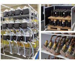
Spare parts are combined into sub-assemblies in order to shorten the time required for the replacement of components such as heat exchangers, compressors, and
