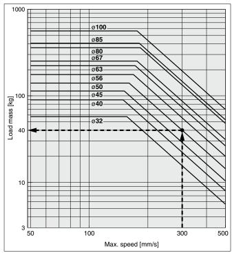
Example) Load limit at the rod end when a ø50 air cylinder is actuated at 300 mm/s Extend upward from 300 mm/s on the horizontal axis of the graph to the intersection point with the line for a 50 mm bore size, and then extend leftward from this point to find the load of 40 kg.
