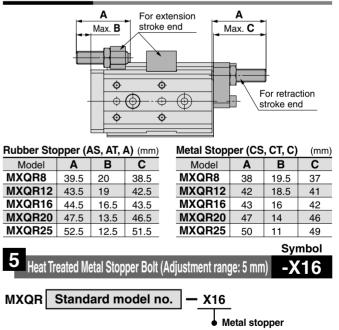
Heat treated chrome-molybdenum steel (SCM435) stroke adjusting thread is used to reduce wearing of metal stopper.
