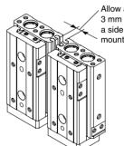
Allow a space of 3 mm or more for a side by side mounting.
