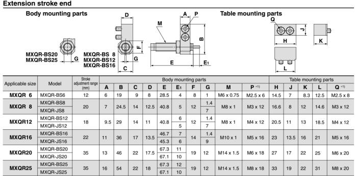
\*1) Size of hexagon socket head bolt \*2) Mounting the adjuster on the left side is also available. For "How to Order", refer to page 3. The outer dimensions are the same as those for mounting the adjuster on the right side.
