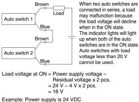
Example: Power supply is 24 VDC Internal voltage drop in auto switch is 4 V.
