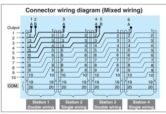
(Refer to the connector wiring diagram.)
