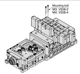
Installation and Removal of Pilot Valve Cover
