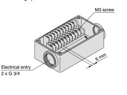
Applicable crimped terminal: 1.25-3S, 1.25Y-3, 1.25Y-3N, 1.25Y-3.5
