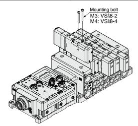
Installation and Removal of Pilot Valve Cover
