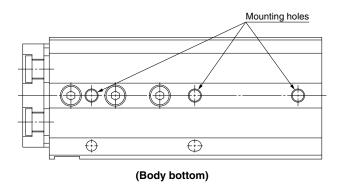
The workpiece mounting position of the end plate is the same as that of the standard product, but note that the max. screw-in depth ("L" dimension) will change.
