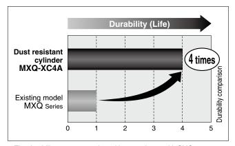
• Lube-retainers are installed on the guide unit and rod cover. This prevents the entry of dust and foreign matter.
