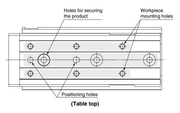
2. When mounting the body, be sure to use all mounting holes on the bottom of the body so that they are not exposed. If there are any unused holes, dust may enter the guide unit, resulting in a reduced service life.
