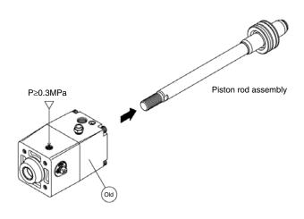
4) Similarly, apply 0.3 MPa or more of compressed air to the unlocking port of the new lock unit, and replace the symposium with the previously mentioned piston rod assembly.
