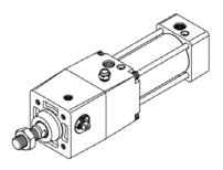
2) Remove the tie-rods, head cover and cylinder tube.
