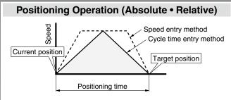
Absolute: The table moves to the target position with reference to the origin position and stops there.
