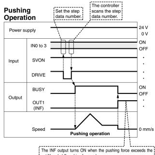
set "threshold" pushing force value. The INF signal turns OFF when the DRIVE signal is turned OFF.
