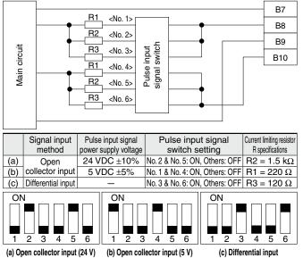
Change the switch in the controller according to the pulse input signal power supply voltage. For differential input, connect the positioning unit using the line driver which is equivalent to DS26C31.
