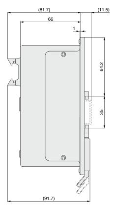
When two or more controllers are used, the space between the controllers should be 10 mm or more.
