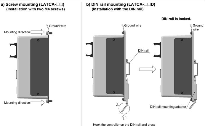
the lever of section **A** in the arrow direction to lock it.
