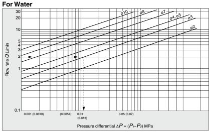
How to read the graph When a water flow of 2 L/min is generated,  $\Delta P$  Approx. 0.013 MPa for a valve with o3 orifice.
